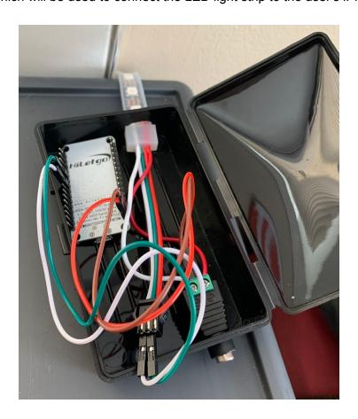
There were many possible choices, but for the current implementation the generic ESP8266 microcontroller is sufficient as this board is capable of handling 5 volts and also has the necessary onboard pins we require: ground, vin, and data - it also has others, which may be used down the line for more advanced features. Above is a photo of our current hardware implementation, excluding the power supply.
