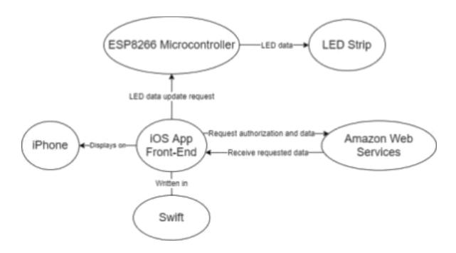
For the Front-End, we will develop the iOS app in the Swift language that is only available on an iPhone. The app will solicit data changes from the LED strip and send them to the ESP8266 microcontroller. The LED light strip is connected directly to the microcontroller so it will receive the LED data and execute the appropriate light pattern.
